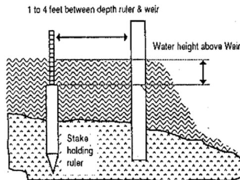
The weir method is more versatile and may prove useful for higher flows. This technique uses a rectangular opening cut in a board or piece of sheet metal set into the brook like a dam. The water is channeled into the weir and the depth is measured from the top of a stake that is level with the edge of the weir and several feet upstream.
