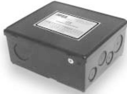
IOTA Engineering Transfer Switches provide automatic power switching between two or three separate 120/240 volt AC input sources, including powercords, onboard generators, onboard inverters, or all three. The ITS will sense the presence of available supplies and automatically select the proper one.
