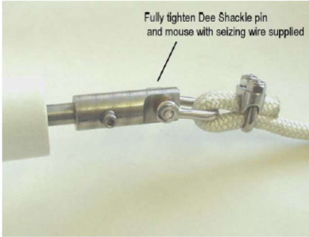
5. Attaching the tow rope to the drive coupling
