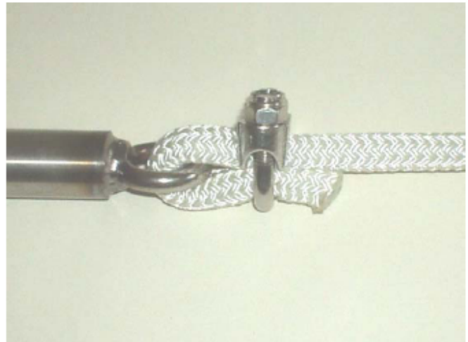
6. Attaching the tow rope to the turbine
